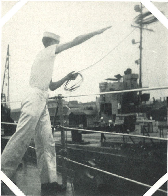
A heaving line with a monkey's fist (weighted end) tossed to dock carries the heavy hawser.
