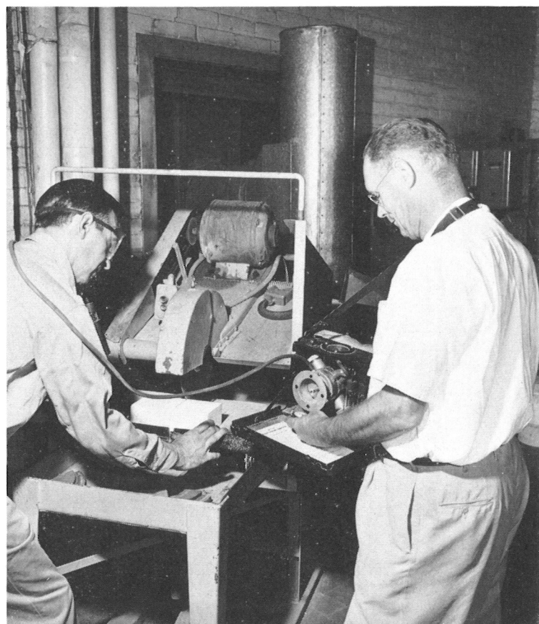
Number of dust particles per cubic foot in breathing zone of Joseph Chilia at Pitney Glass Works masonry saw is checked by R. S. Mackie of Chemical Products Works.
